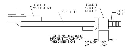
**NOTE:** Belt deflection or movement should be approximately 1/4" when measured at mid-point between pulleys.
